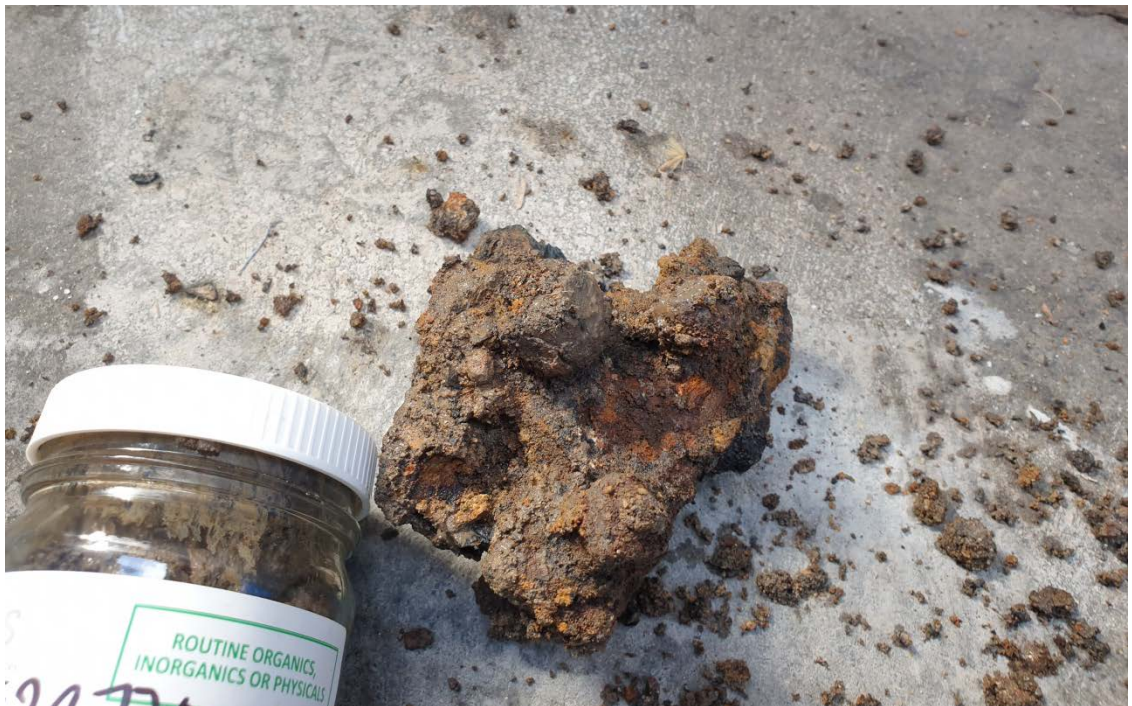
Photograph 4: Image of large scrap metal, heavily deteriorated, found within shallow fill material at borehole location 'BH4' (01.09.20).
